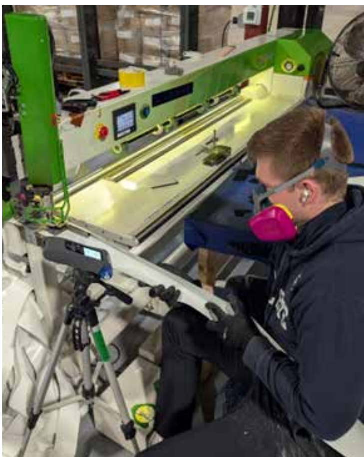
Figure 1. A Renegade Plastics employee outfitted with proper PPE hot air welding PVC.
